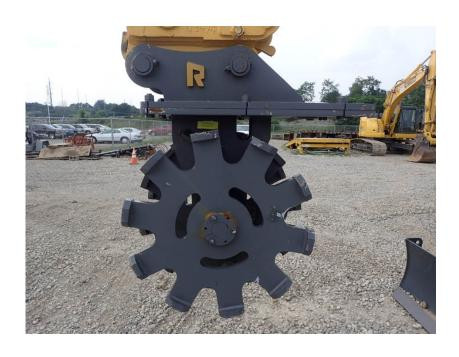
Attachments: 2021 Rockland W124-3 24" Tamper Foot Compaction
