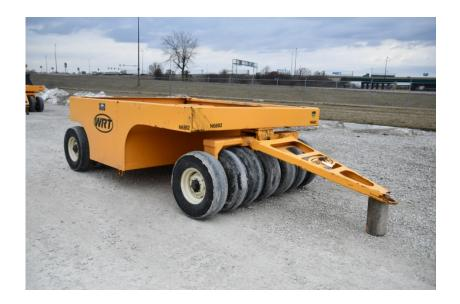
**Compaction Equipment - Smooth Drum**: 2020 WRT PT15W Tow Behind Pneumatic Roller
