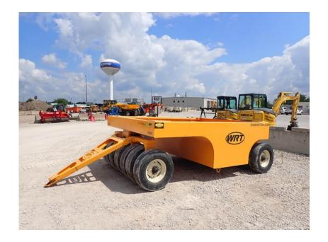
**Compaction Equipment - Smooth Drum**: 2020 WRT PT15W Tow Behind Pneumatic Roller
