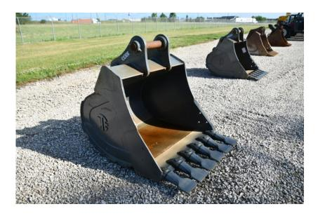
Attachments: TAG 48" SK210/SK235SR/SK230SR/SK270SR Excavator
