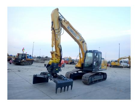
Excavator: 2021 Kobelco SK170LC-10 w/Heavy Counterweight
