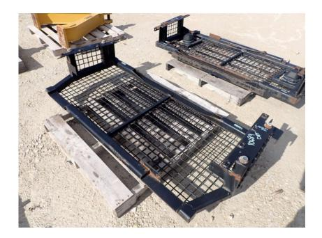
Attachments: CAT D8T Rear Window Cab Protection Screen Stock Number: JT007
