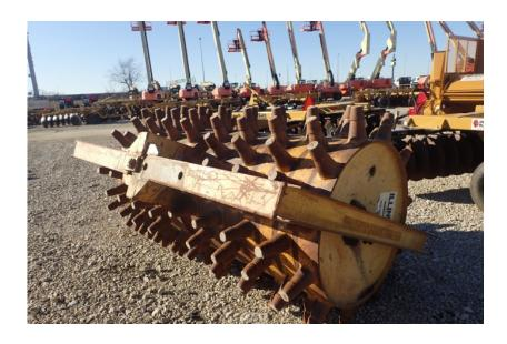
Compaction Equipment - Padfoot: Wabco 56" Pull Type Padfoot Drums Stock Number: 11033
