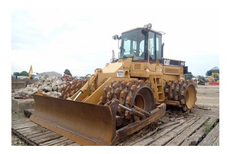
Compaction Equipment - Padfoot: 2006 Cat 815F Padfoot Roller
