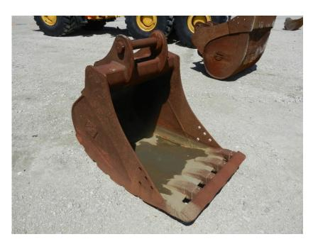
**Excavator Bucket Attachments: SK140-SK170**
