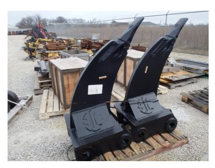
**Excavator Frost Ripper Attachments:** SK210-SK235
