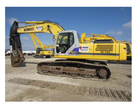
Excavators With Shears 2nd Member: Kobelco SK350 LC
