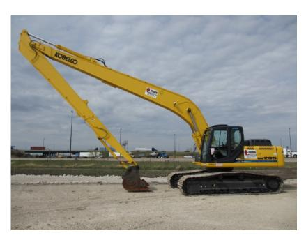
Kobelco Long Reach Excavators: Kobelco SK300 LC
