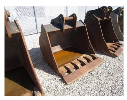
**Excavator Bucket Attachments: SK210-SK260**
