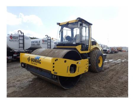
Compaction Equipment - Smooth Drum: 2019 Bomag BW211D-5
