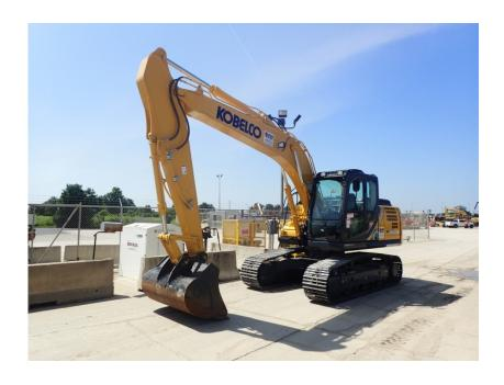
Excavator: 2019 Kobelco SK170LC-10 w/Heavy Counterweight
