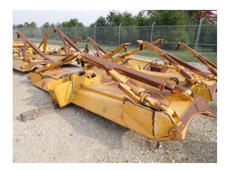
Attachments: Rockland D6T LGP Angle Blade and C Frame
