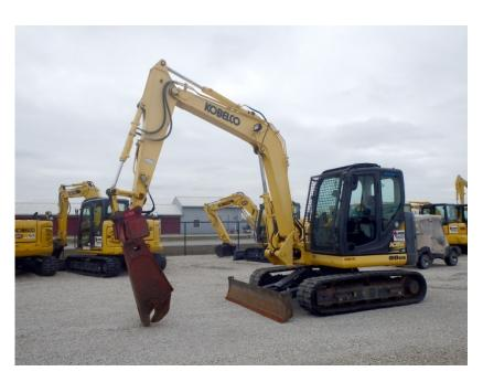
Excavators With Shears 3rd Member: Kobelco SK85CS
