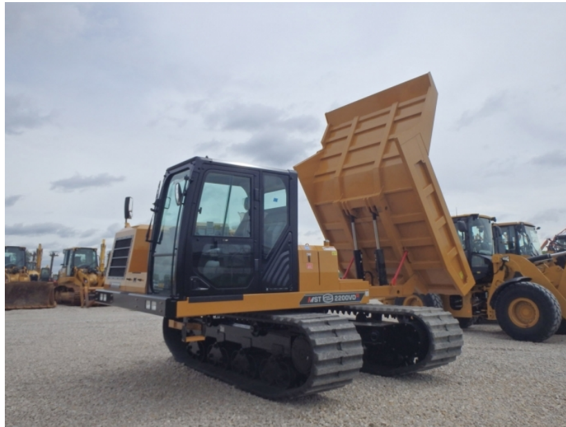
Off Road 360 Degree Rotating Rubber Track Dumpers: Morooka MST2200VDR 360 Degree Rotation
