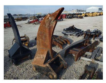
**Excavator Frost Ripper Attachments:** SK300-SK350
